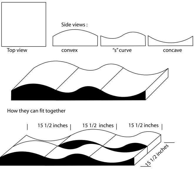
Wave modules can be made as half modules (7 3/4" x 15 1/2") and put together to form square modules 15 1/2" square.
